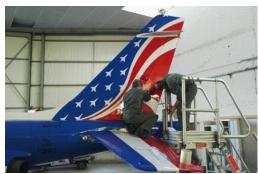
After painting the drifts, the mechanics finish the decoration by affixing the identification number of each aircraft. © PAF
