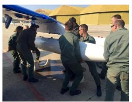
Installation of additional fuel cans under the Alphajets wings, necessary for long distance transport. © PAF
