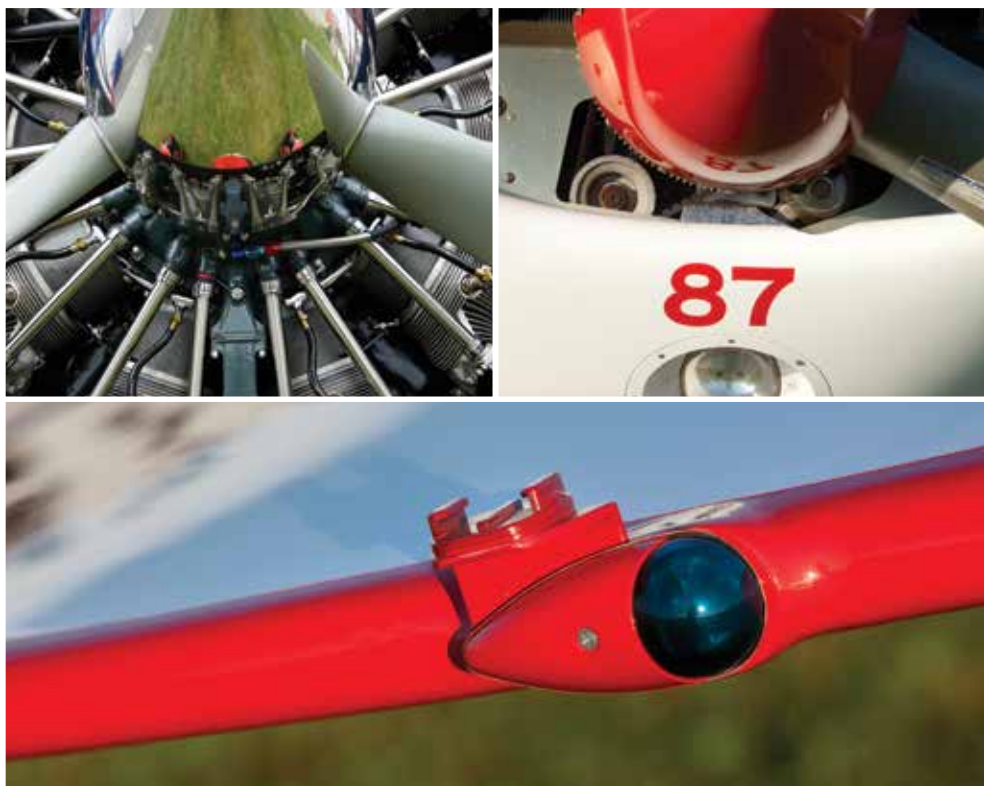
Upper left: Hartzell spinner and R-985 of the Jet Waco. Upper right: CAP 10B spinner and hand-lettered serial number. Bottom: CAP 10B wingtip light.
